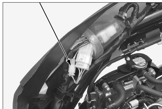
CONECTOR 2P DO SENSOR CKP
